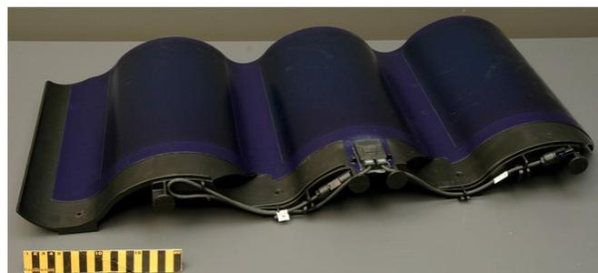
Photovoltaic roof tile
